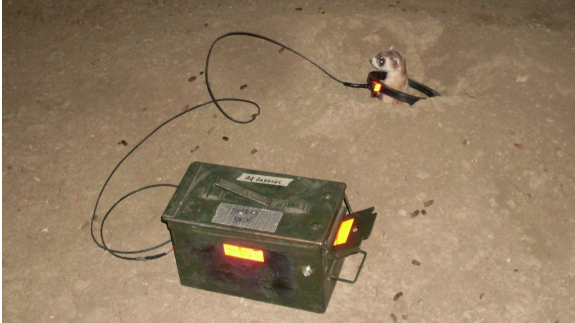
Figure 29. Black-footed ferret passing through a ring reader in Saskatchewan, Canada. The reader is configured for long-term field deployment with a sturdy case and batteries that can last for 2 weeks. Photo by Travis Livieri.
