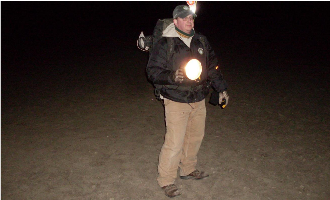
Figure 53. Striker 170 handheld spotlight attached to BP9SLA Kit Battery Bag powered by 9 amp-hour sealed lead acid battery. This configuration with a 30 watt bulb lasts 4-6 hours of continuous spotlighting. Photo by Travis Livieri.
