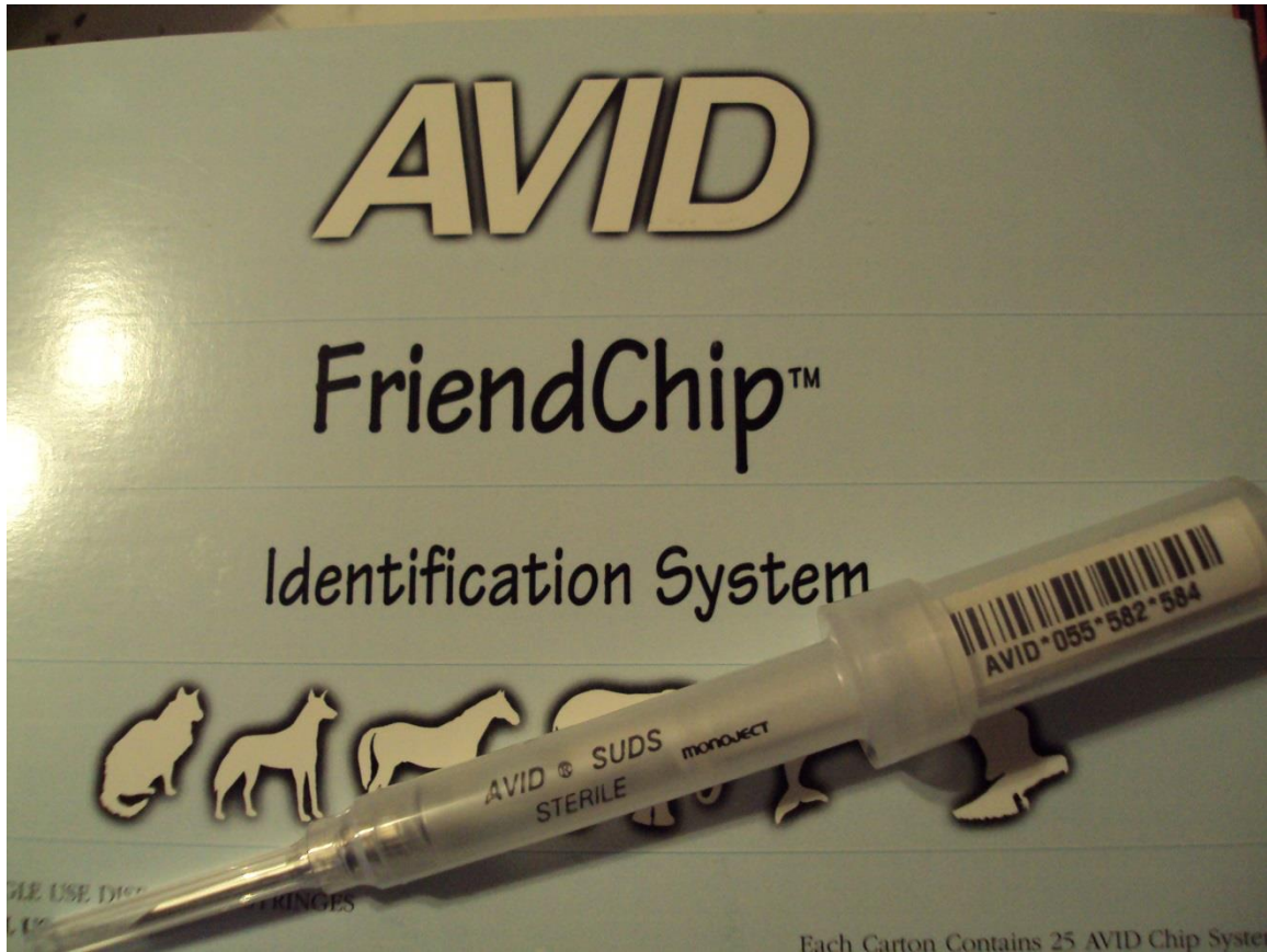
Figure 56. FriendChip (125 kHz) PIT tag manufactured by AVID in the Single Use Disposable Syringe (SUDS). Photo by Travis Livieri.
