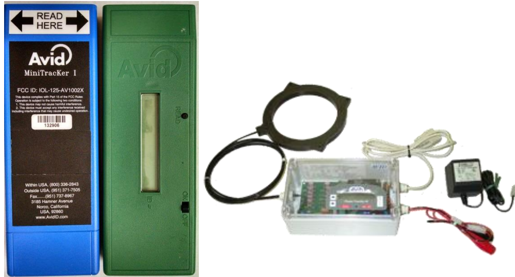
Figure 57. AVID Minitracker hand-held PIT tag microchip reader (left) and AVID Industrial Stationary Reader (right).
