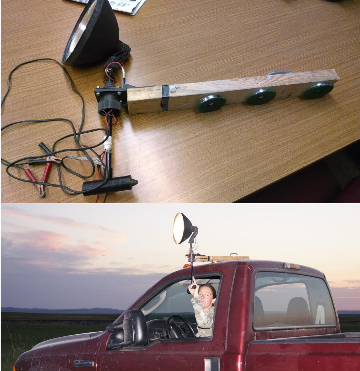
Figure 49. RM240 Blitz with RC225 T-bar grip and RCEXT hinge mounted to a 2"x4" and magnetic mounts for easy use on top of a vehicle. The power cord with alligator clips attaches directly to the vehicle battery. Other configurations include mounting to thick foam, rather than wood, to provide flexibility on the curved roof of a vehicle. Some newer vehicles may have an aluminum body making magnet-mounts useless. Photos by Travis Livieri.
