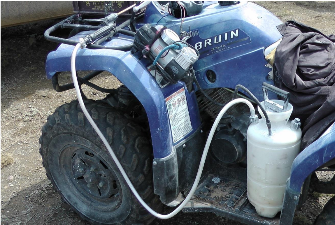
Figure 63. Birchmeier DR-5 powder duster with compressed air valve connected to a 12-volt air pump. Photo by Travis Livieri.
