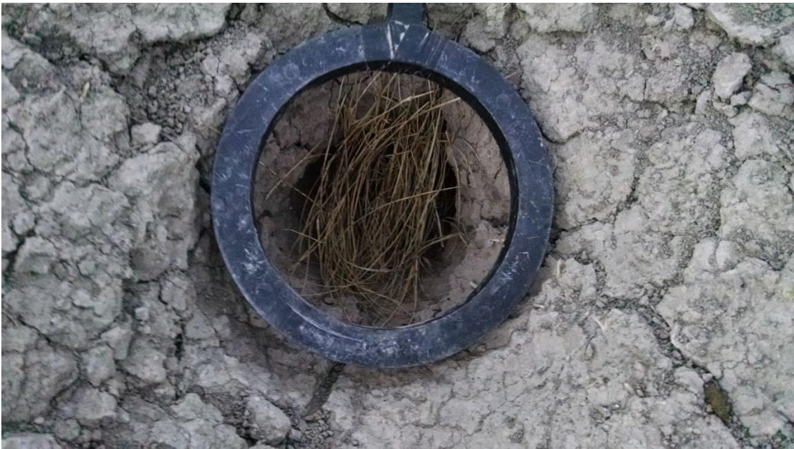
Figure 28. A shallow grass plug in a prairie dog burrow with a ring reader. If a ferret passes through the reader then the grass will be obviously moved and can help determine if the ferret does not have a PIT tag. Photo by Travis Livieri.
