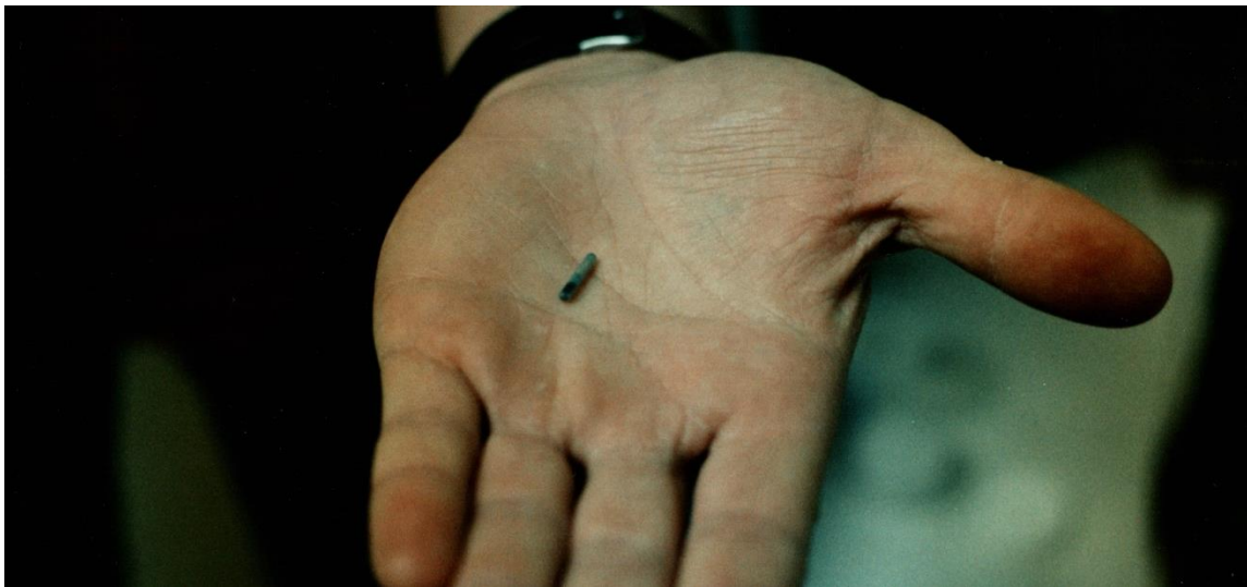
Figure 26. Passive integrated transponder (PIT) tag manufactured by AVID. Photo by Travis Livieri.
