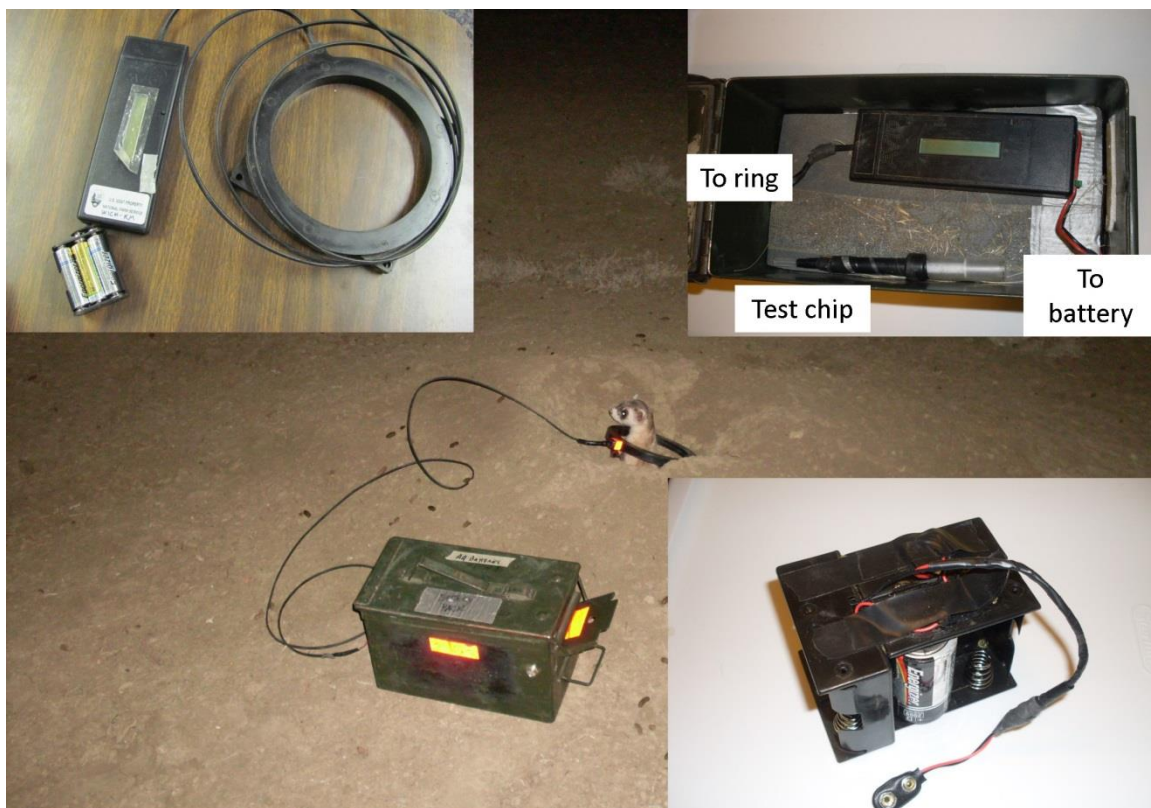
Figure 58. AVID Minitracker with 6” coil modified for long-term field use. Upper left is the configuration that comes from the manufacturer with a 9-volt (6 AA battery) power pack for longer battery life. Upper right, a military style ammunition box was used for protection from the elements with the ring coil threaded through the front of the box and a 9-volt modified battery pack below (6 D battery) and shown being used in the field (primary picture). This modified 6 D-cell battery configuration provides up to 2 weeks of continuous use in cold conditions.
