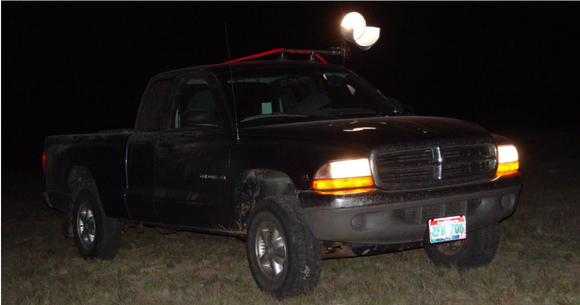
Figure 50. RM240 Blitz with RC225 T-bar grip and RCSBC Suction Bar Kit. The suction cups allow easy attachment to any vehicle. A ratchet strap can be used to keep the suction bar in place while surveying. Other configurations include replacing the metal bar with thin wall conduit across the width of the vehicle and mounting a spotlight on each side of the vehicle. Photo by Travis Livieri.
