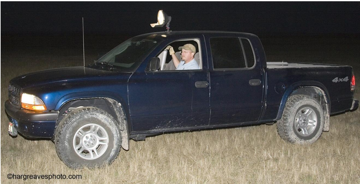
Figure 51. RM240 Blitz with RC225 T-bar grip mounted through the roof of a pickup truck. A 2" hole is required for installation. This configuration is preferred by most biologists. Photo by Diane Hargreaves.
