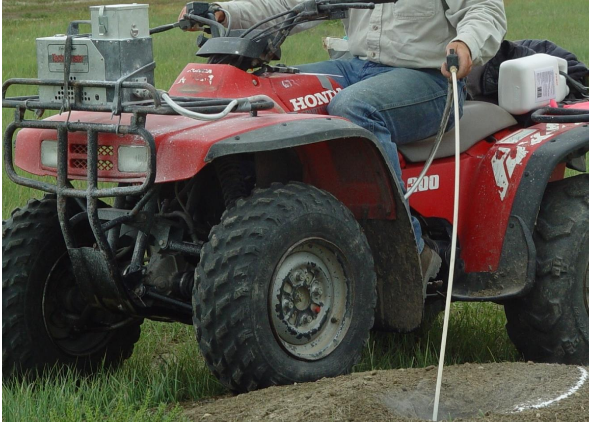
Figure 61. Techniduster (model shown is discontinued) manufactured by Technicide. Photo by Travis Livieri.
